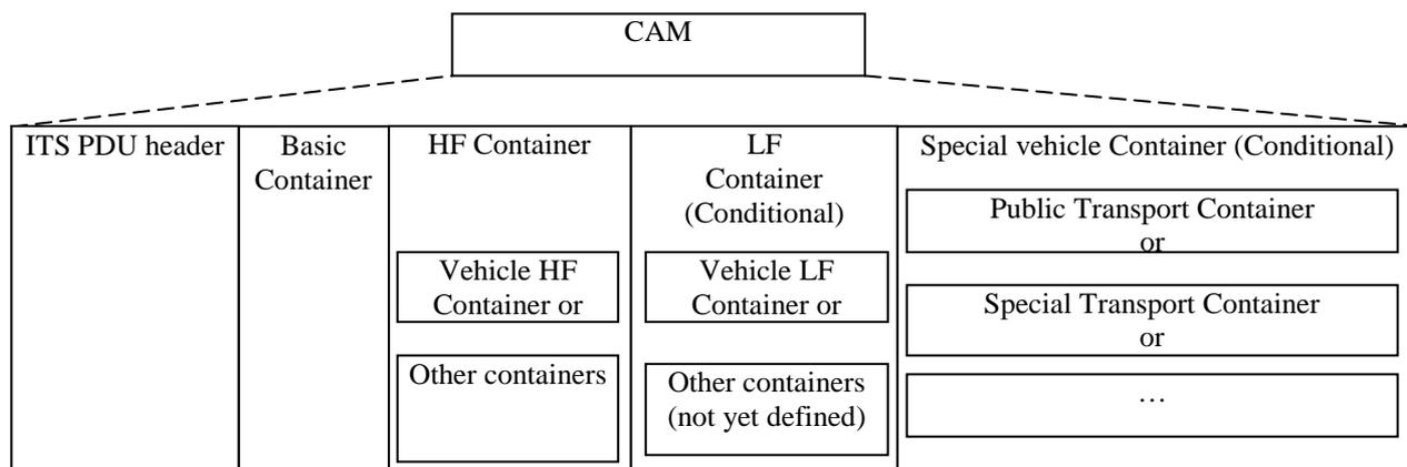
Figure 4: General structure of a CAM
