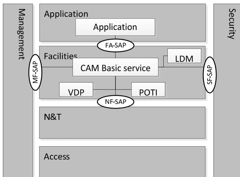
Figure 1: CA basic service within the ITS-S architecture
